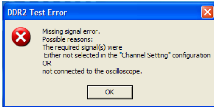
Figure 108 Missing Signal Error Message
